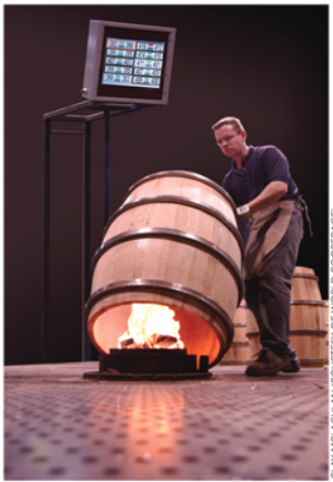
A cooper toasts a barrel with the aid of computer technology. The sensor that feeds data to the computer monitor aids the cooper in creating and replicating custom barrel profiles for white wines.
